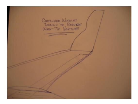
This design will improve airflow and reduce drag, indeed a morphing leading edge surface could reduce drag by another 22%.
