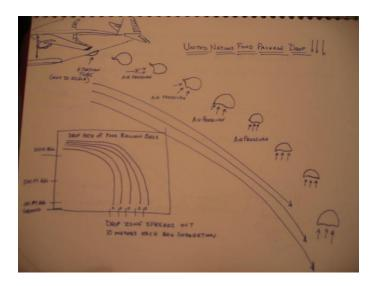
Each package contains a 3-day food package, these drops are delivered directly over the emergency area, without the need for large pallet drops. Below is the Mechanism Design, which uses ram-air to fill the prepackaged containers.
